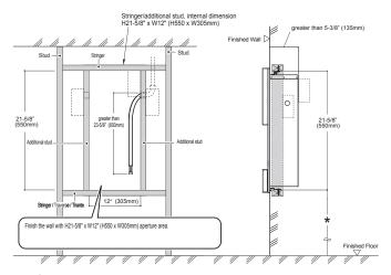
★ Recommended mounting bracket (lower) heights from floor For general users: 31-1/4"(795mm) For users in wheel chairs: 23-7/8"(607mm)
