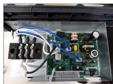
Power circuit board (JT-37P2H)
