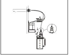
10.Push the soap tank into the mounting brackets. Make sure the soap pump plate is under the pushing shaft before you put back the soap tank so the soap dispenser can work properly. Plug in the AC adapter to complete the installation.
