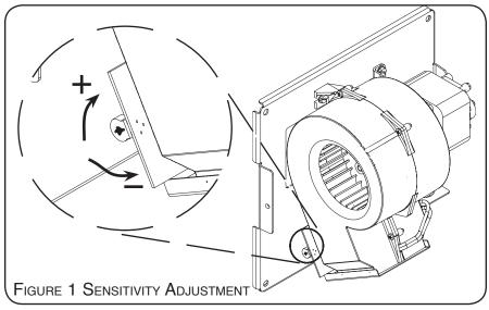
Remove the cover and check to see that the fan revolves freely. Check and replace motor, if required.
